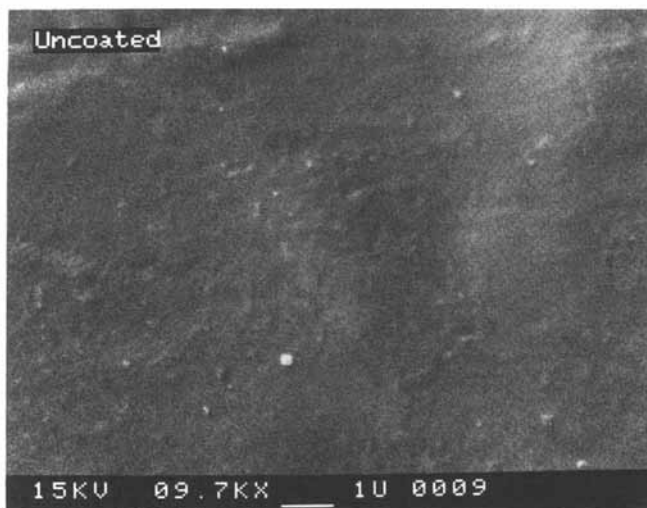
Figure 10(b). Electron micrograph of the untreated LDPE film surface at 9.7 \times 10^3 magnification.
